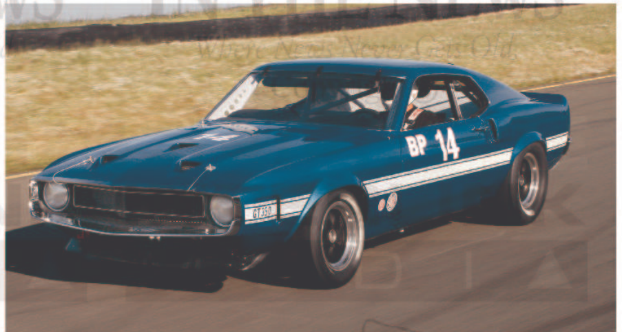
▲ This car wore American 200S wheels at times during its racing career, and Goering was lucky to find a period correct 15x8-inch set in magnesium. Restored by Vintage Engineering's Ray Franklin, they're mostly for show—any hard driving will be done on newer wheels with more reliable metallurgy.
