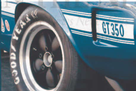
▲ This car wore American 200S wheels at times during its racing career, and Goering was lucky to find a period correct 15x8-inch set in magnesium. Restored by Vintage Engineering's Ray Franklin, they're mostly for show—any hard driving will be done on newer wheels with more reliable metallurgy.
