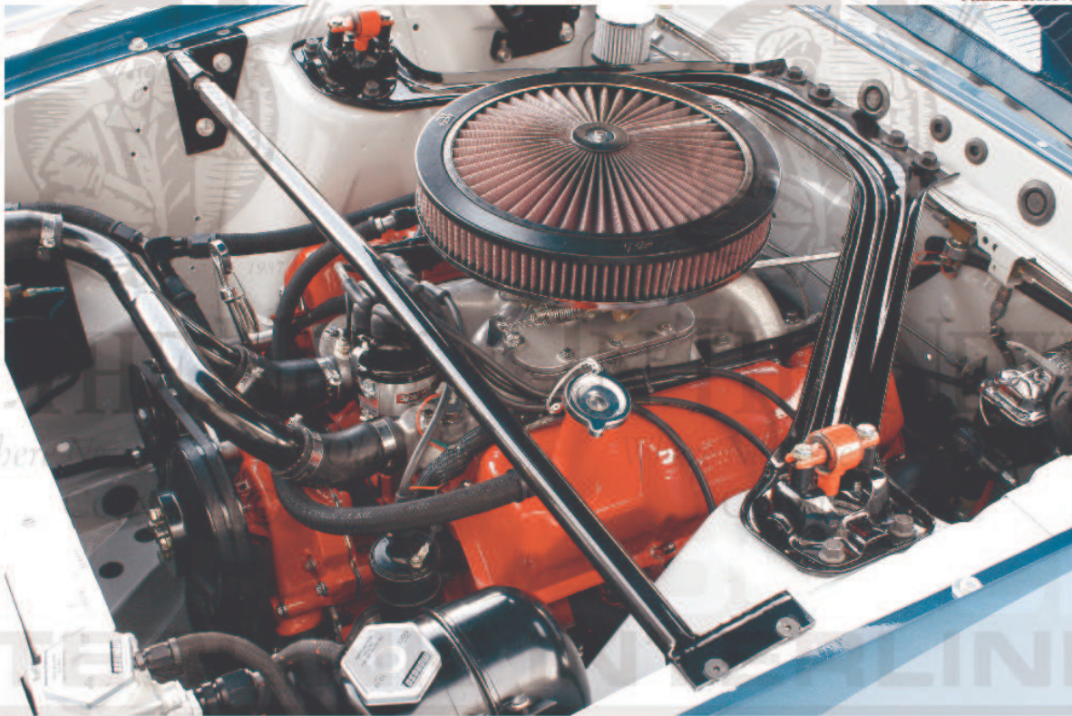
▲ Red seems an odd choice for a Ford engine of the '60s, until you learn that it was the color of choice for Doane Spencer builds. The stout Boss 302 was assembled by Skip Govia, and features a Bud Moore mini plenum that Spencer worked over.
